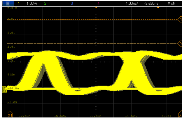
Figure 8.4 NSi8210N Eye diagram of output signal at 200Mbps
